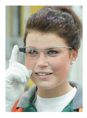
oogle Glass is the brand name of a mini computer worn on the head and equipped with an optical display that is mounted at the periphery of the field of vision on one of the temple arms. As well as projecting information on the display, other information can also be combined with photos taken by the integrated digital camera. Furthermore, data can be downloaded directly from the internet and sent.
